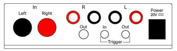
Make all connections whilst the amplifier is disconnected from the mains. Take care to connect the left and right channels correctly. The right channel is usually marked red, the left channel black or white. Make sure the polarity of the connection is correct at each end of the cables.
